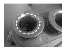
(990-950-SE) Properly oiling your filter with No Toil Oil and thoroughly greasing the foam lip of the filter, secure it to the lower base plate by locking in the left side filter tab (Red) underneath the black base plate tab and rocking it down onto the ¼ turn tabs.
