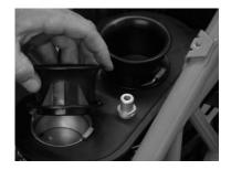
**(990 only)** Plug in the white temp sensor and route the wires above and away from any and all moving parts.
