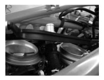
(990-950-SE) Secure the base plate above the "X" rings making sure they are seated into the machined grooves of the bottom of the plate. Re attach the velocity stacks to lock the base plate down. The ¼ turn silver tabs on the base plate should face the right of the motorcycle.
