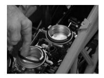
(990-950-SE) Upon installation of the plate, you may need to re route the crankcase breather slightly differently to accommodate going underneath the throttle cable mount on the forward throttle body. Warning: Make sure this DOES NOT interfere with any moving parts
