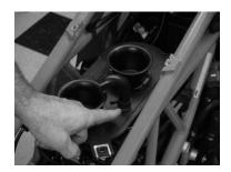
(950 SE only) On SE versions only you must cut down the velocity stacks in order to fit the "Dome" style filter. Any apparent downsides of this are quickly negated by overall surface filtration gain and this set up has been extensively tested to a high level of rider satisfaction.
